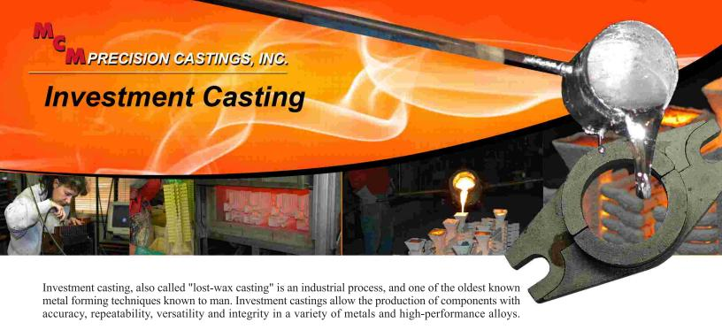
The investment casting process is generally used for small castings, but has been used to produce items of much larger size and dimension. The process is generally more expensive per unit than die casting or sand casting, but with lower equipment cost. Investment casting can produce complicated shapes that would be extremely difficult to impossible with die casting. Yet like the die casting process, investment casting requires little surface finishing and only minor machining.
